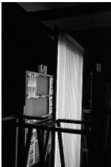
Figure 11: Light-fading unit at IPI
