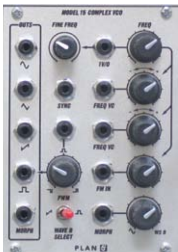
FIG. 4: The Plan B Model 15 Complex VCO is a beefy-sounding oscillator that gives you voltage control over the waveshape at the Morph output.
