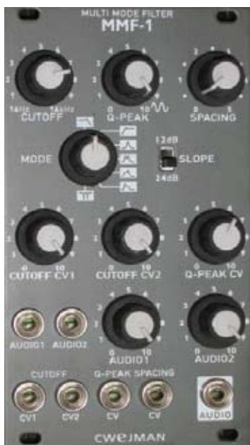
FIG. 5: The Cwejman MMF-1 multimode filter offers three dual bandpass modes, each of which gives you two sine tones when the filter goes into resonance.
