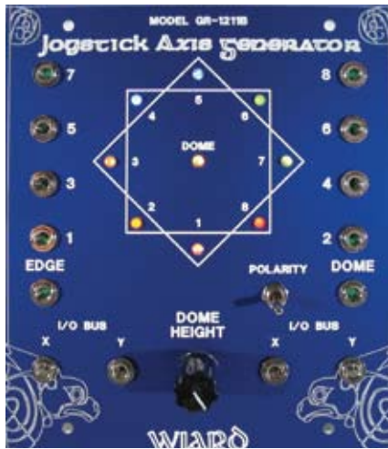
FIG. 8: Wiard's Joystick Axis Generator lets you control ten voltage inputs using a single joystick controller.
