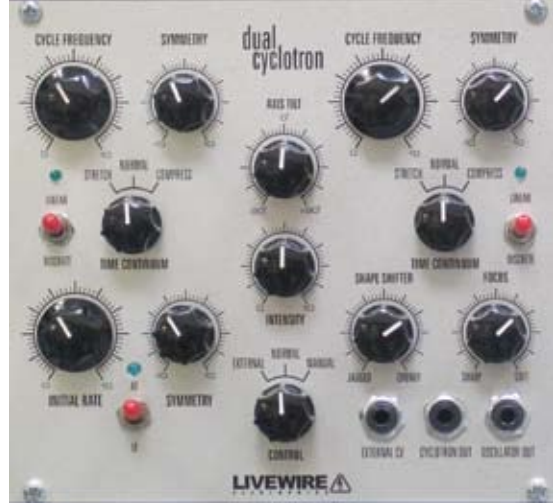
FIG. 3: In the Livewire Dual Cyclotron, three oscillators interact with each other, sometimes in seemingly mysterious ways.
