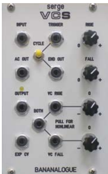
FIG. 1: The Bananalogue Serge VCS can be used as an EG, an envelope follower, and an oscillator.
