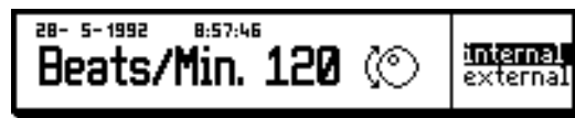
“Clock” window: Rotate the dial to modify the Tempo and escape with EXIT.
